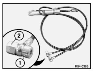
Plug hose connections for hydraulic cylinder:
